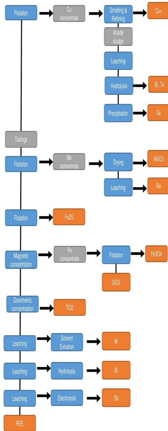
Figure 2. Qualitative diagram for a technological process for the recovery of metals from tailings and copper concentrates (Silva, et al., 2017), (Habashi, 2017).
