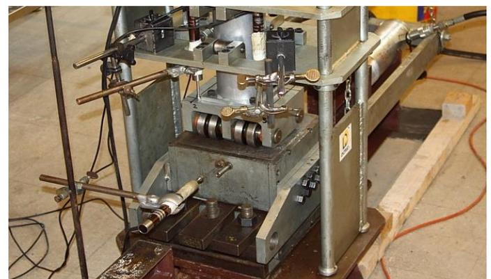
Figure 3. Direct shear tests equipment.
